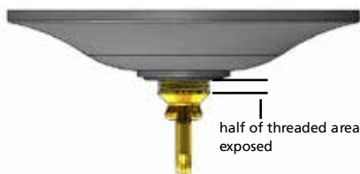
Drawing 2 Canopy Adjustment
